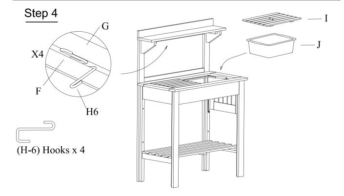
Place Plastic Sink (J) into position on Table Panel (H) as shown.
