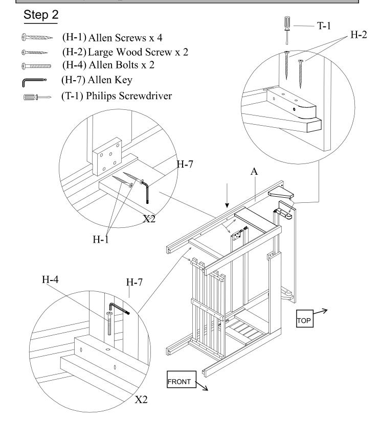
Secure Left Panel (A) to the assembly from Step 1 as shown. Secure the top using 2 Large Wood Screws (H-2) and a Phillips Screwdriver (T-1) (not included).
